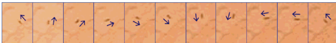
Figure 3. Snapshots of a typical rotary motion of a Si/Pt nanorod. The time interval between two adjacent frames is 0.1 s. In the experiment, both the clockwise and counterclockwise rotations have been observed due to the random orientations of the nanorods in the solution.
