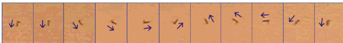
Figure 6. Snapshots of a typical rotary motion of an L-shaped Si/Pt nanorod. The time interval between two adjacent frames is 0.4 \text{ s} . For this case, we also observed both the clockwise and counterclockwise rotations.
